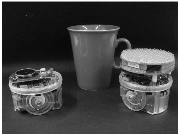
(a) The e-puck and an e-puck with the see-puck display attached standing next to an ordinary coffee mug.
